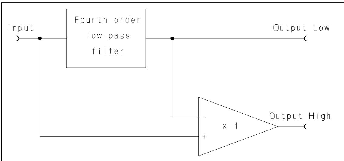
**Figure 22:** Schematic diagram of subtraction filter.
