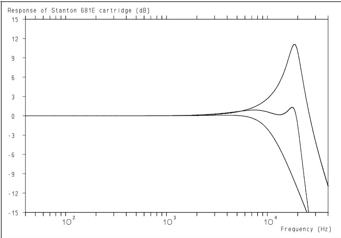
**Figure 11:** Response of Stanton 681E cartridge. Lower curve = electrical response, upper curve = mechanical response, middle curve = overall response.
