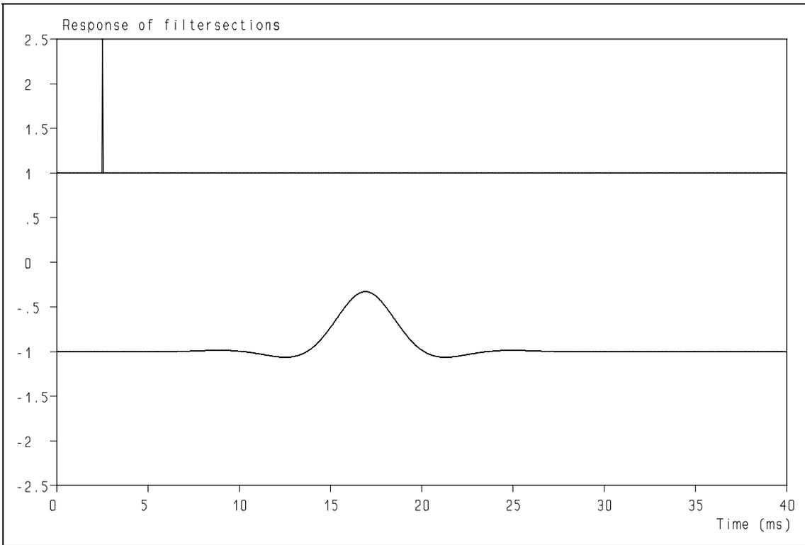
**Figure 29:** Example of phase-linear causal low-pass filter with "pre"-ringing.
