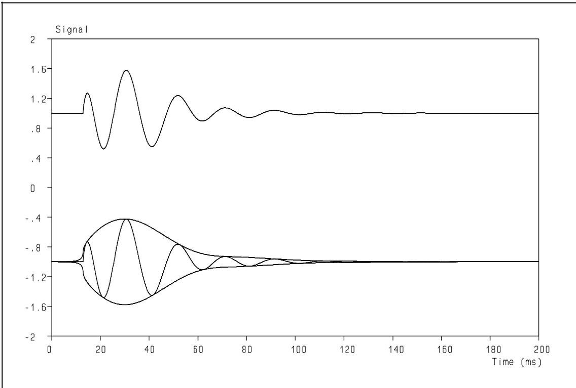
**Figure 37:** Response of a bass-reflex system to a simulated kettle-drum signal showing the envelope as well.
