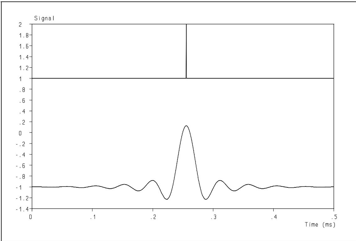
**Figure 15:** Impulse response of a CD reconstruction filter.
