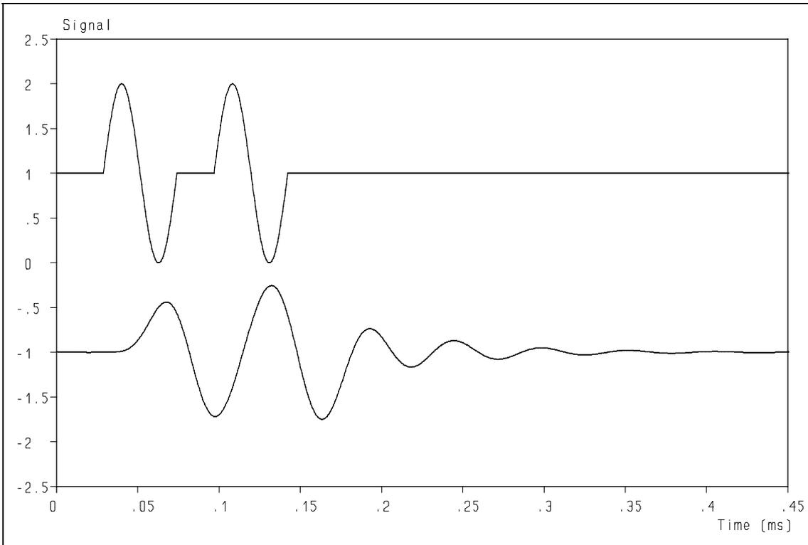
**Figure 12:** Response of a moving magnet cartridge to a complex signal.
