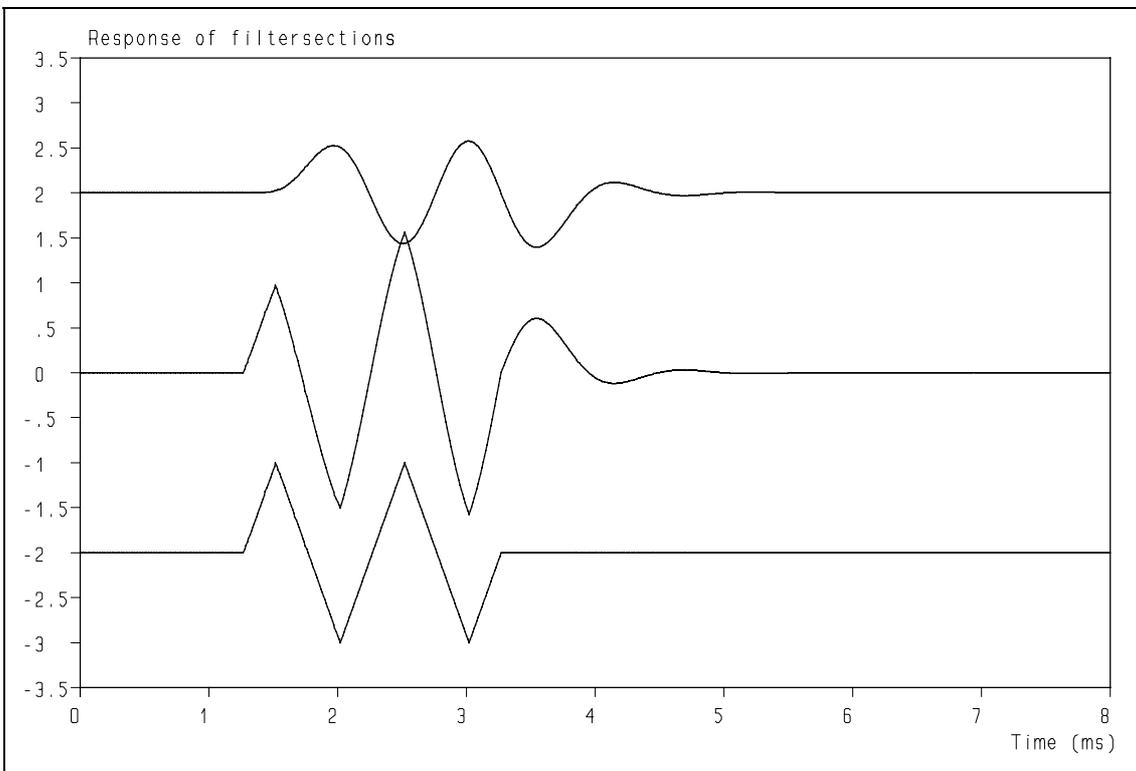
**Figure 26:** Response of fourth order Butterworth low-pass filter (upper trace), its complement (centre) and the summed response (lower trace).
