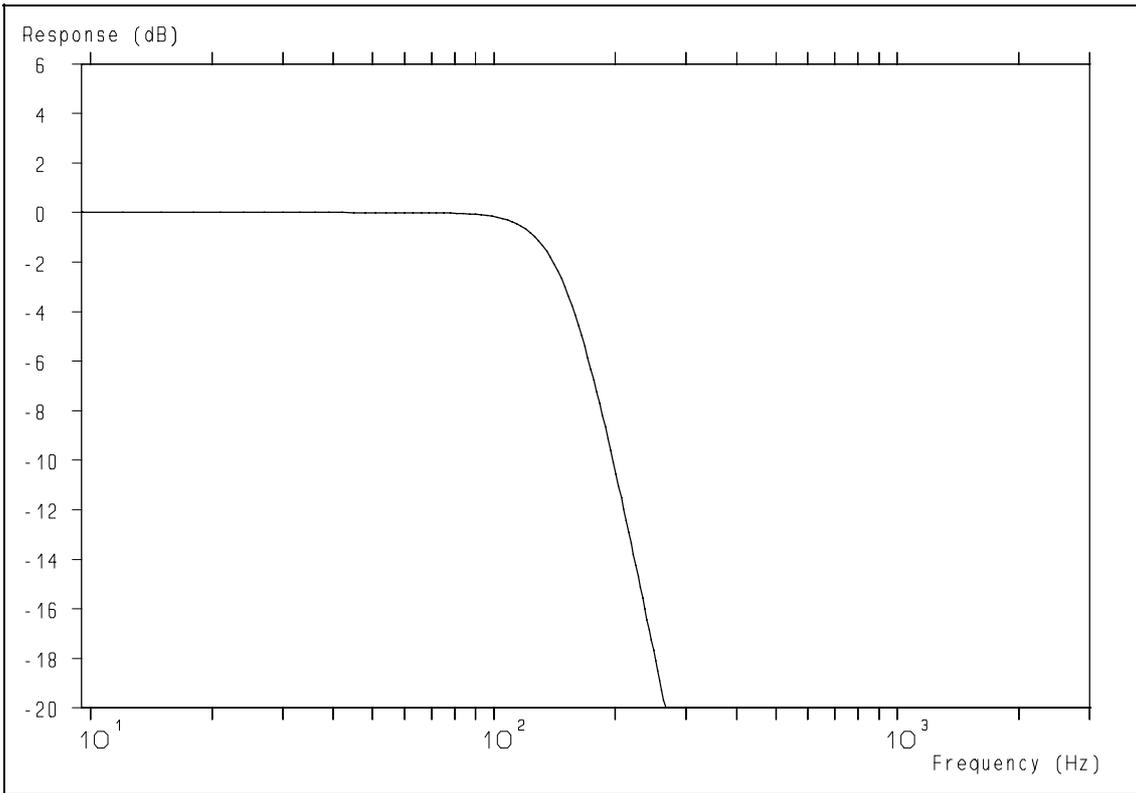
**Figure 23:** Response of fourth order Butterworth low-pass filter of 150 Hz.
