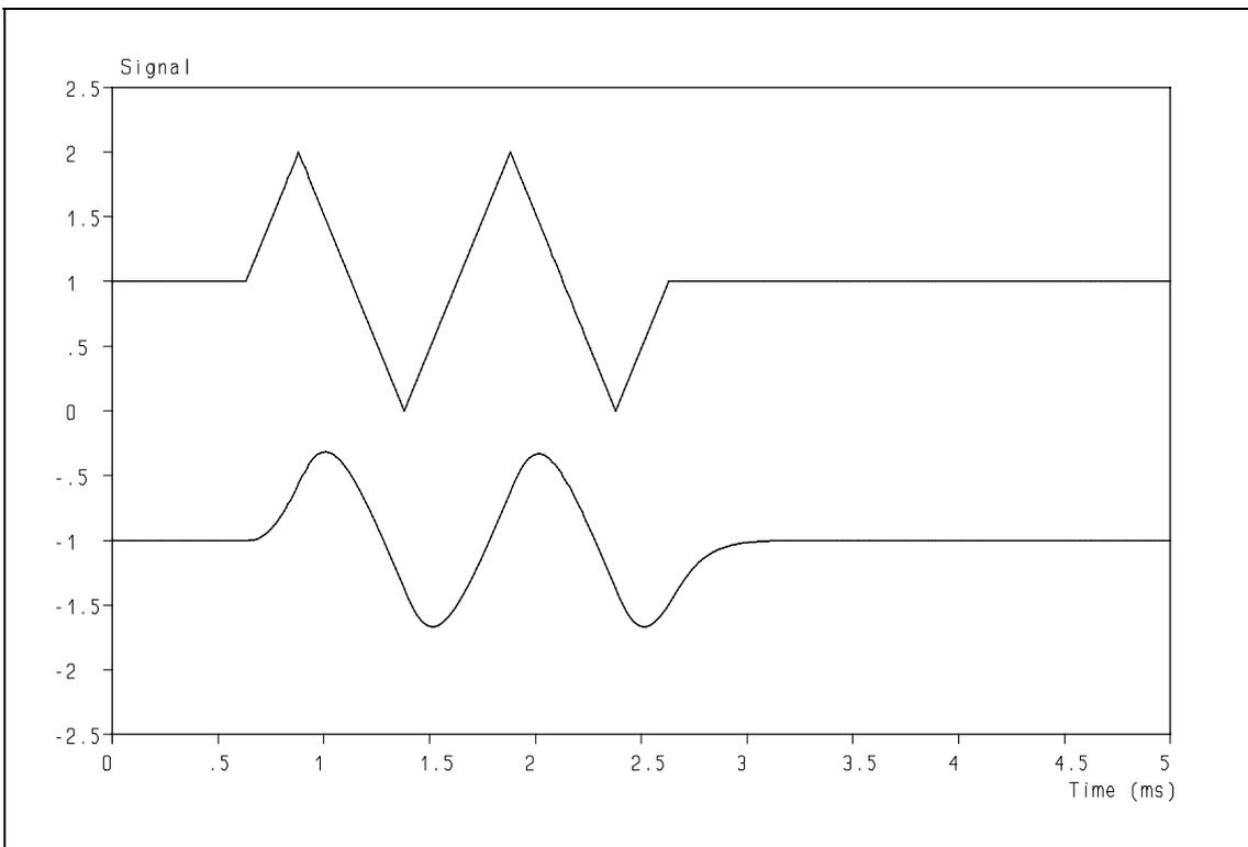
**Figure 32:** Response of low-pass section of phase-correct analog filter (second order).
