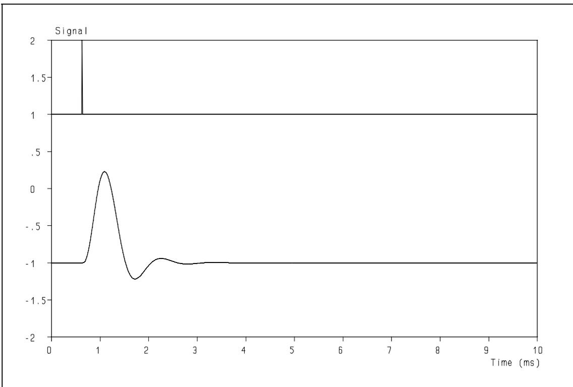
**Figure 6:** Impulse response of a 4<sup>th</sup> order Butterworth filter.
