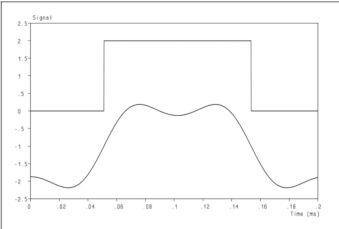
**Figure 16:** Step response of a CD reconstruction filter.
