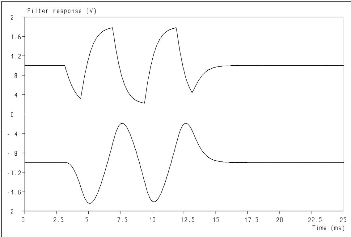
**Figure E-1:** Calculated response of analog filter sections. Compare with fig. D-2.
