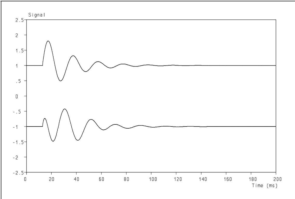
**Figure 36:** Response of a bass-reflex system to a simulated kettle-drum signal.
