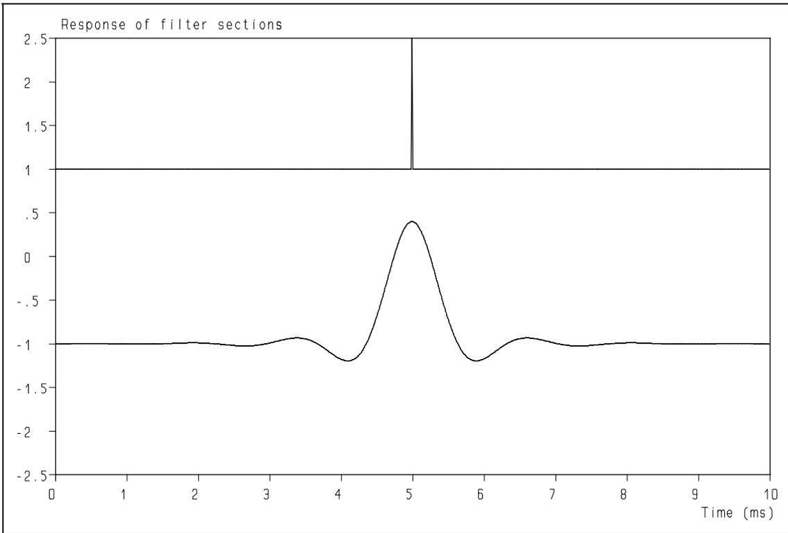
**Figure 27:** Impulse response of a 6<sup>th</sup> order digital Butterworth low-pass filter.
