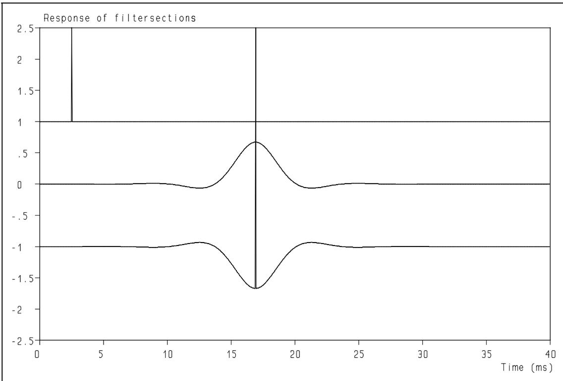
**Figure 30:** Example of phase-linear causal filters with "pre"-ringing which require the two loudspeaker units to create complete silence before the onset of the sound. (N.B. The peak at 17 ms. is part of the lowest trace)
