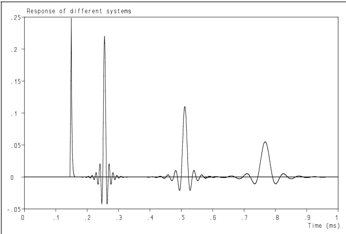
**Figure 18:** Responses (from left to right) of a DSD, a 192 kHz, a 96 kHz and a 48 kHz system on a -6 dB block input of 3  $\mu$ s duration and an amplitude of 0.25 (from ref. 7).
