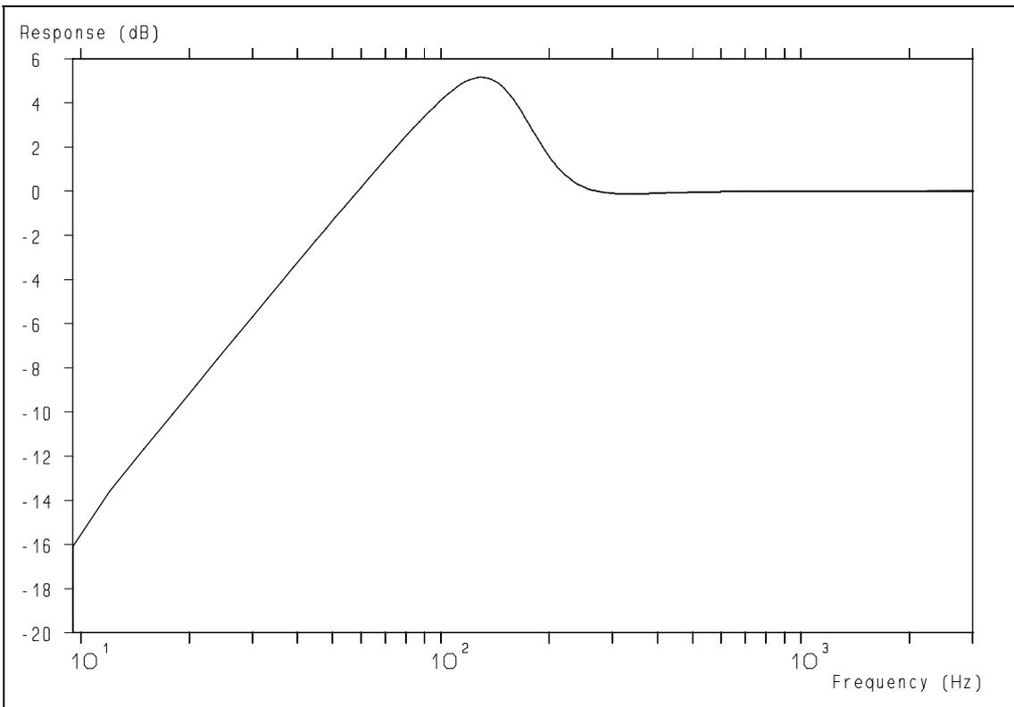
**Figure 24:** Response of the complement of the fourth order Butterworth low-pass filter of 150 Hz.
