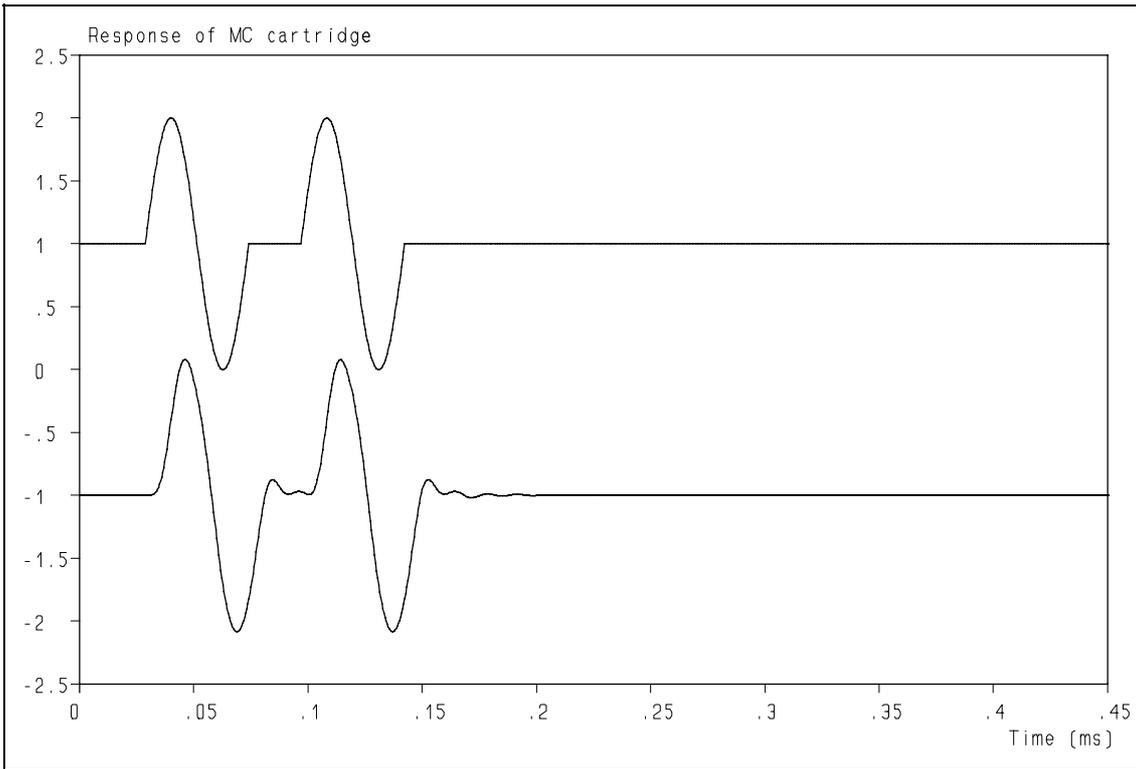
**Figure 13:** Response of a moving coil cartridge to a complex signal.
