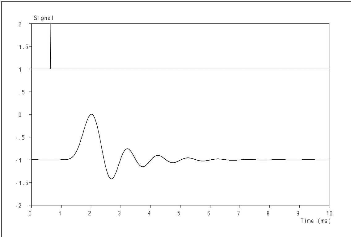
**Figure 7:** Impulse response of a 12<sup>th</sup> order Butterworth filter.
