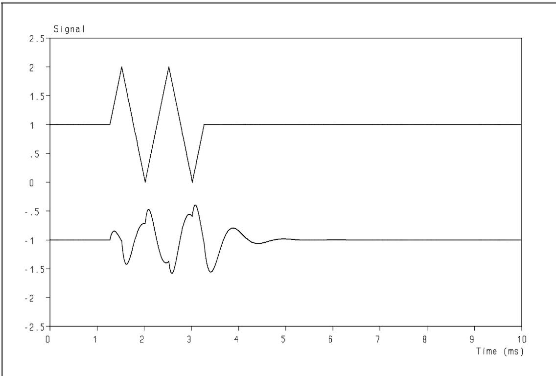
**Figure 20:** Response of 4<sup>th</sup> order Butterworth high-pass filter to a complex signal.
