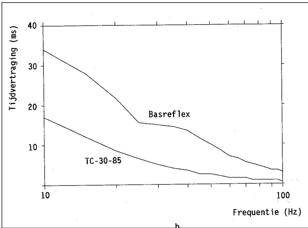
**Figure 42:** Delays of two different woofer systems, the bass-reflex and the electronically compensated woofer in an acoustic box. For more details, see text.
