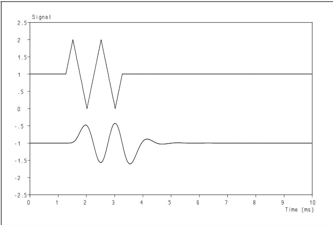
**Figure 19:** Response of 4<sup>th</sup> order Butterworth low-pass filter to a complex signal.
