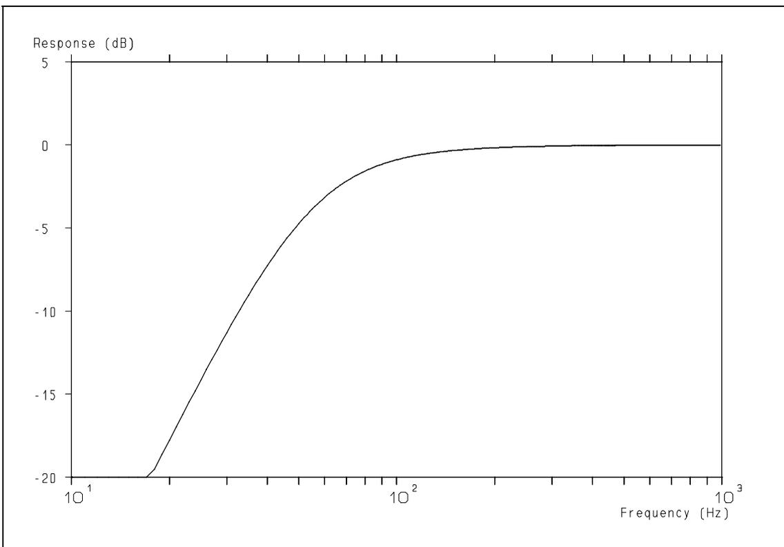
**Figure 38:** Response of the woofer in its acoustic box. Note the absence of a resonance peak, Q approx. 0.63.
