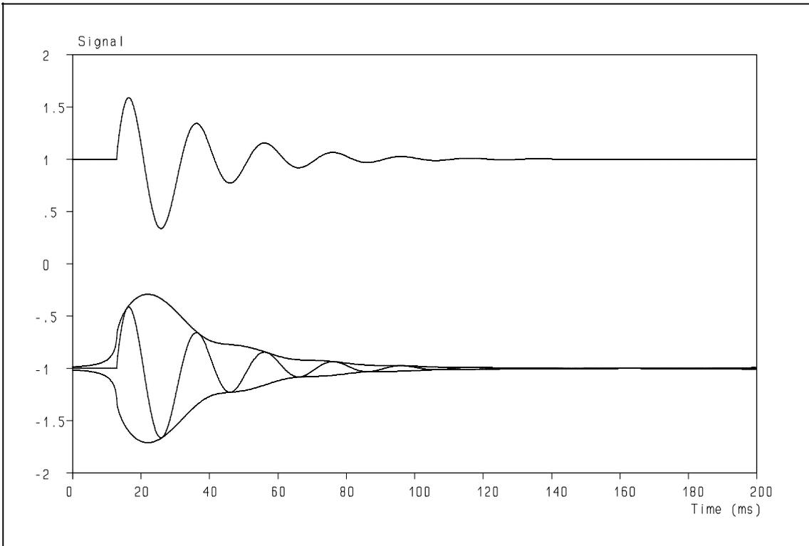
**Figure 41:** Response of an ABC-2 compensated woofer system to a simulated kettle-drum signal showing the envelope as well.
