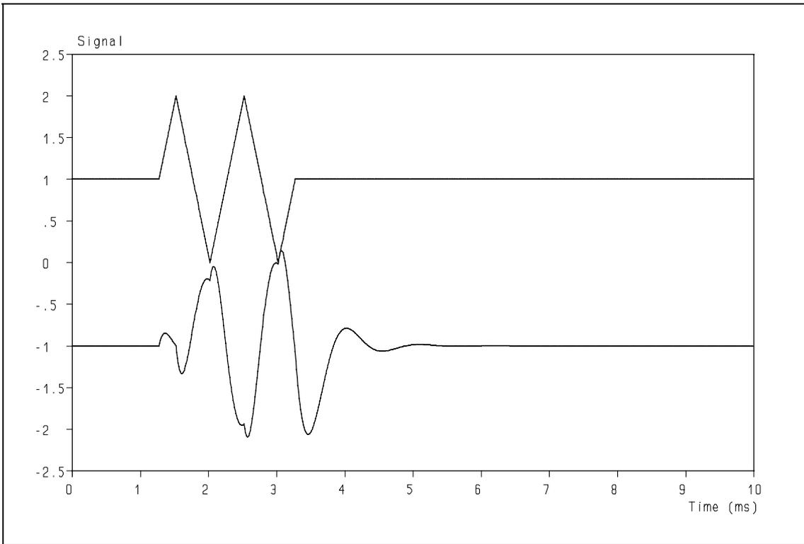
**Figure 21:** Combined response of 4<sup>th</sup> order Butterworth low and high-pass filters to a complex signal.
