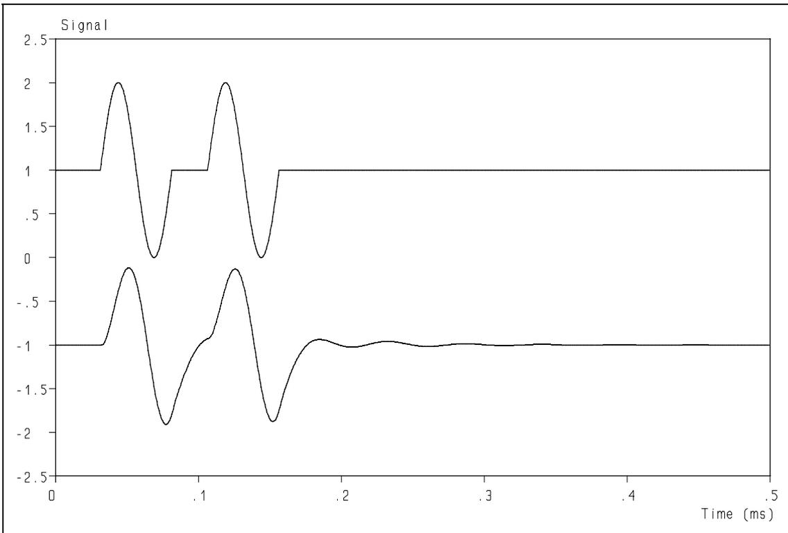
**Figure 14:** Response of a moving magnet cartridge to a complex signal after compensation.
