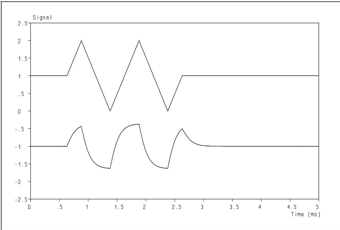
**Figure 33:** Response of high-pass section of phase-correct analog filter (less than first order).
