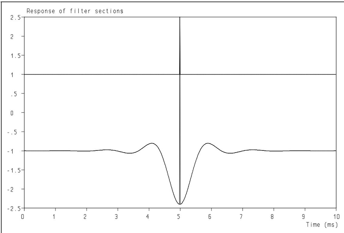
**Figure 28:** Impulse response of the complement of a 6<sup>th</sup> order digital Butterworth low-pass filter. (N.B. The peak at 5 ms. is present in both upper and lower trace)
