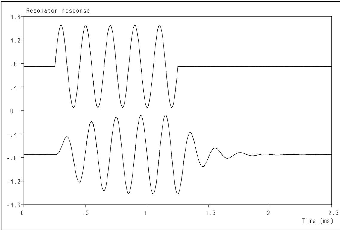
**Figure 35:** Resonators are slow because they need time to start and time to decay.
