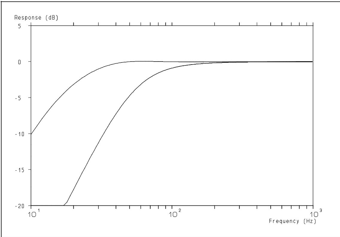
**Figure 39:** Response of the woofer in its acoustic box without (lower curve) and with compensation (upper curve) using the ABC-2.
