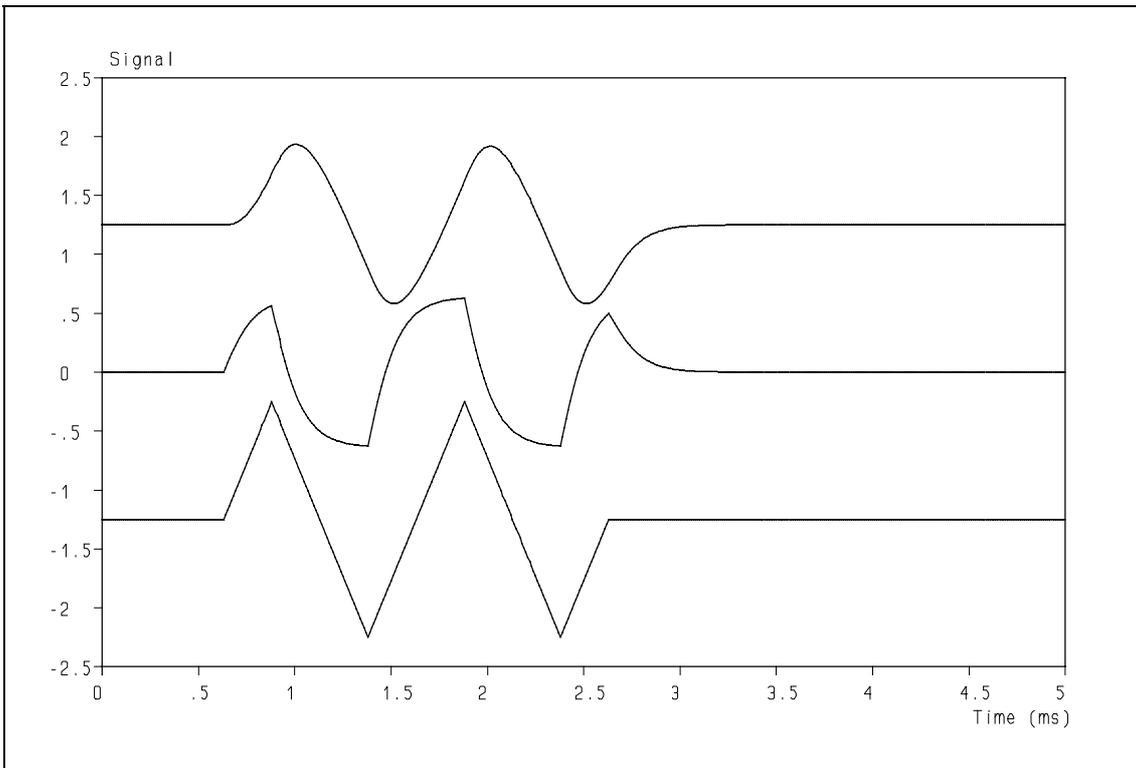
**Figure 34:** Combined response of low and high-pass sections of phase-correct analog filter.
