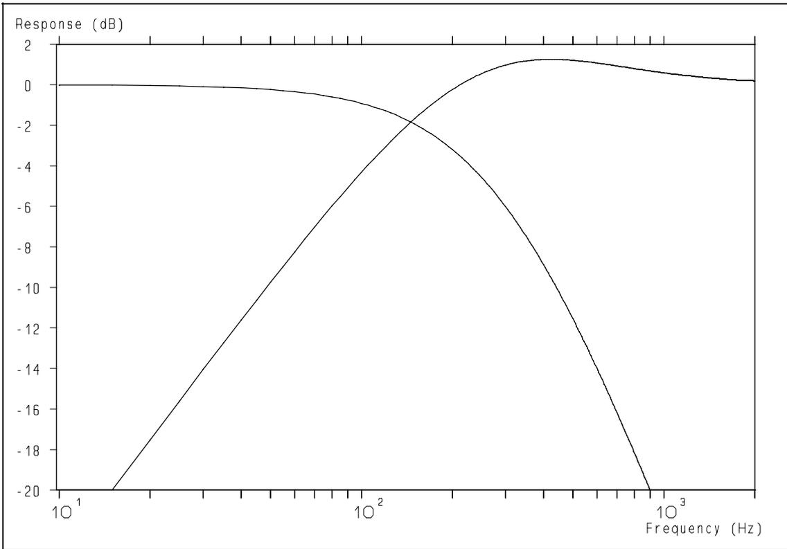
**Figure 31:** Response of a second-order analog low-pass filter and its complement to create a time-correct overall response.
