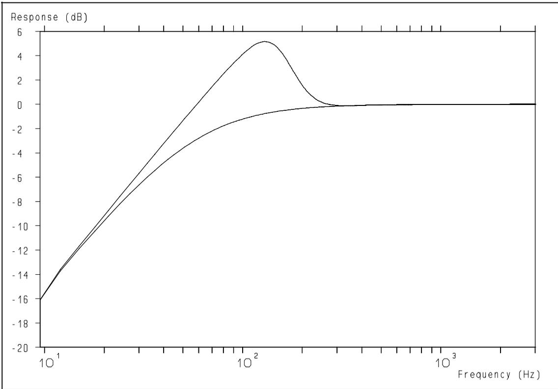
**Figure 25:** Response of complement of fourth order Butterworth low-pass filter of 150 Hz and a first-order high pass filter of 57 Hz.
