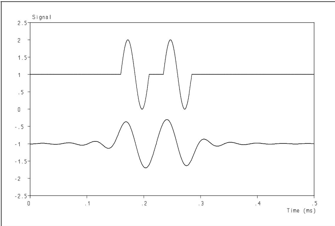
**Figure 17:** Response of a CD reconstruction filter to a complex signal.
