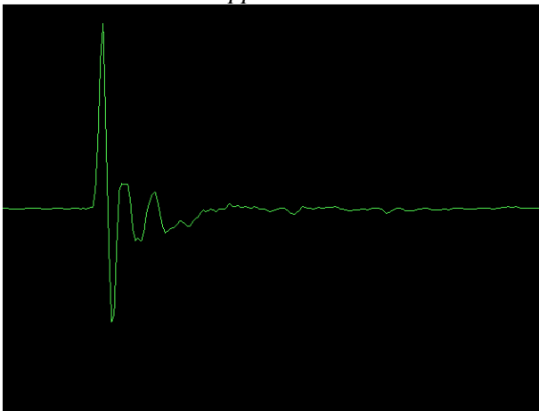
Figure 22: Impulse response of the Condenser Measurement Microphone and tweeter before any correction has been applied.
