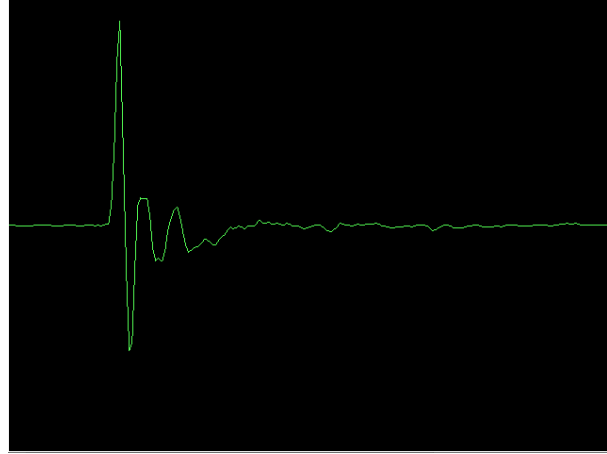
Figure 22: Impulse response of the Condenser Measurement Microphone and tweeter before any correction has been applied.
