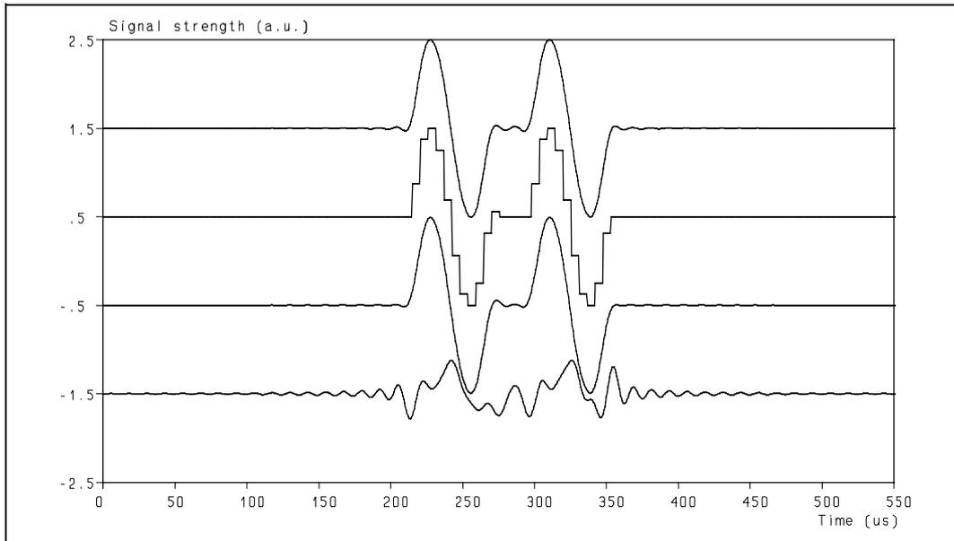
**Figure 12:** Signals in the digital signal processing. Sampling frequency 180 kHz, anti-aliasing and reconstruction filtering at 80 kHz.
