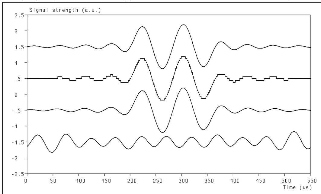
**Figure 7:** Signals in the digital signal processing. Sampling frequency 1800 kHz.
