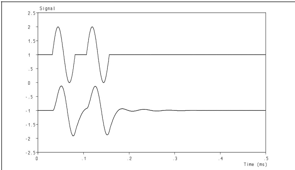
**Figure 3:** Response of a moving magnet cartridge to a complex signal after compensation.
