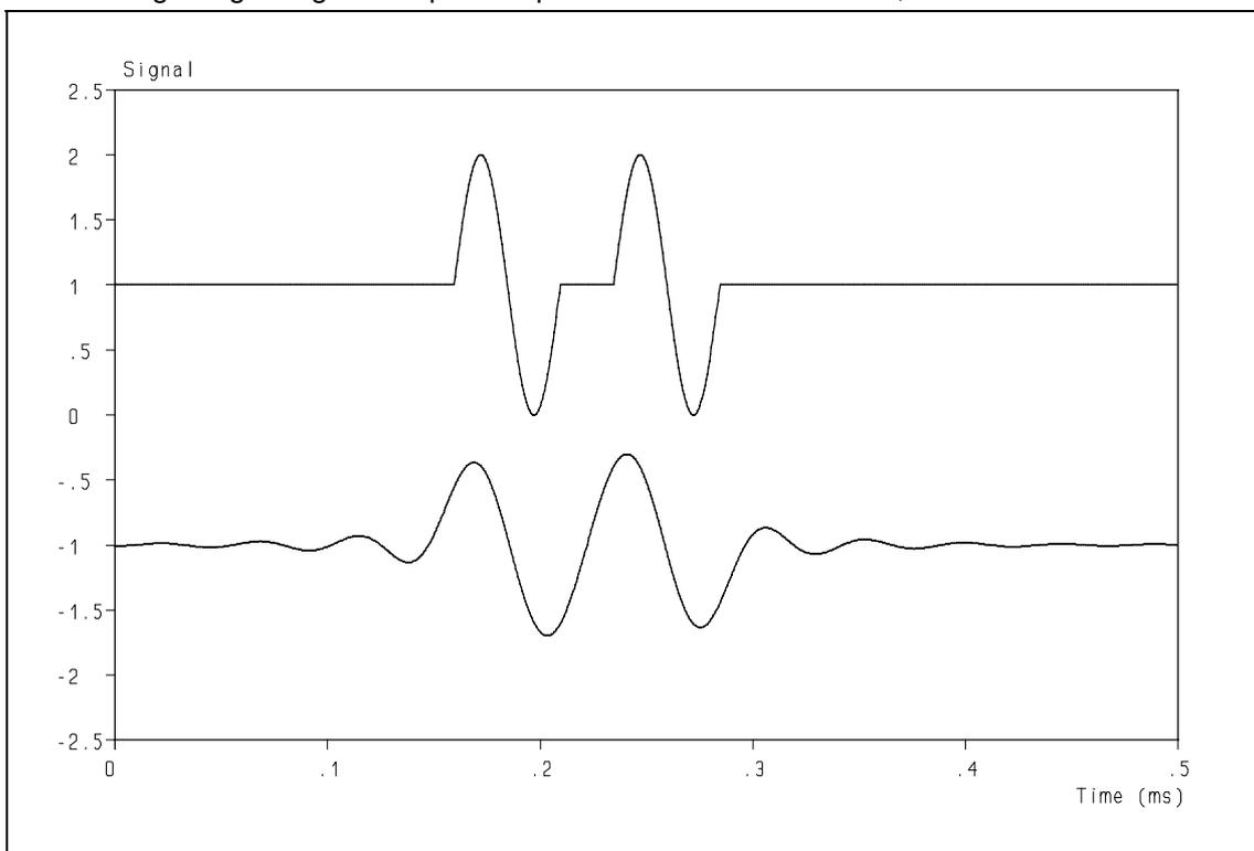
**Figure 6:** Response of a CD reconstruction filter to a complex signal.
