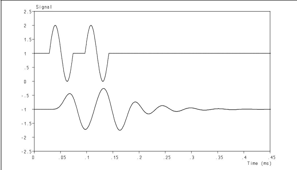
**Figure 2:** Response of a moving magnet cartridge to a complex signal.
