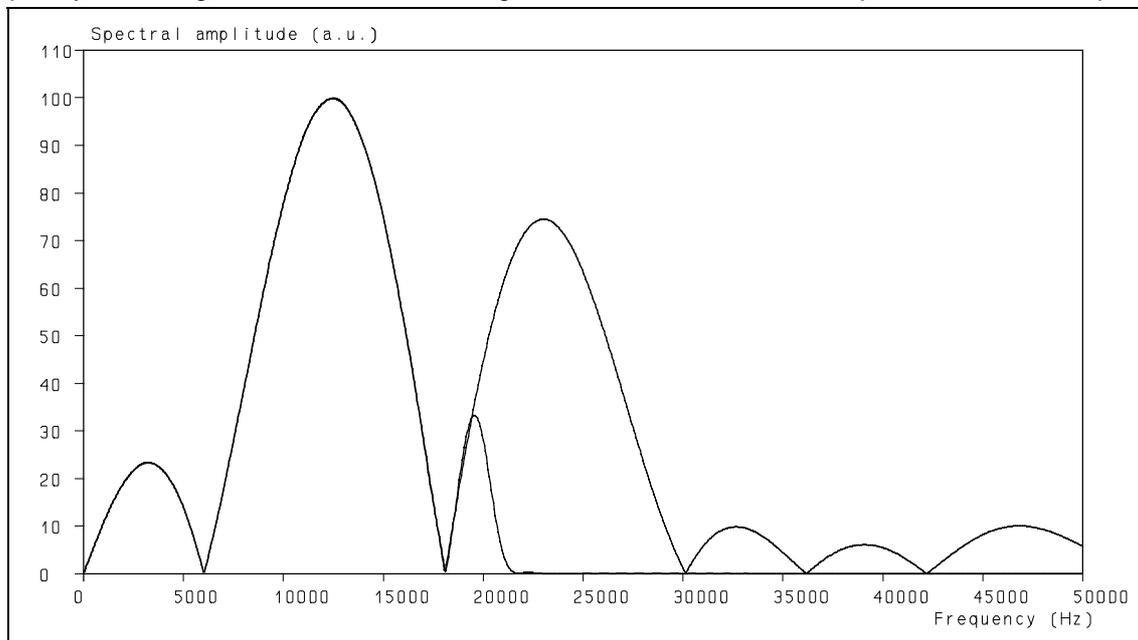
**Figure 9:** Spectra of the input signal (upper trace) and the output of the anti-aliasing filter (lower trace). Note that the frequency of the individual single sine waves (18 kHz) is absent in the spectra!
