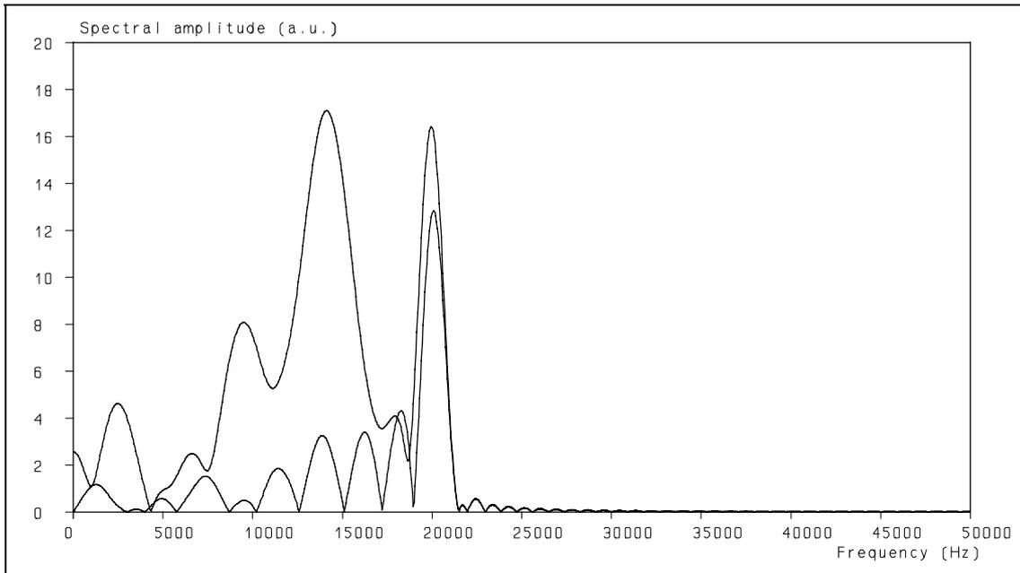
**Figure 10:** Spectra of the noise signal of the 44.1 kHz sampling (upper trace) and the 1800 kHz sampling, using the same anti-alias and reconstruction filtering. Note the vertical scale (compare with fig. 9, the units are the same!).
