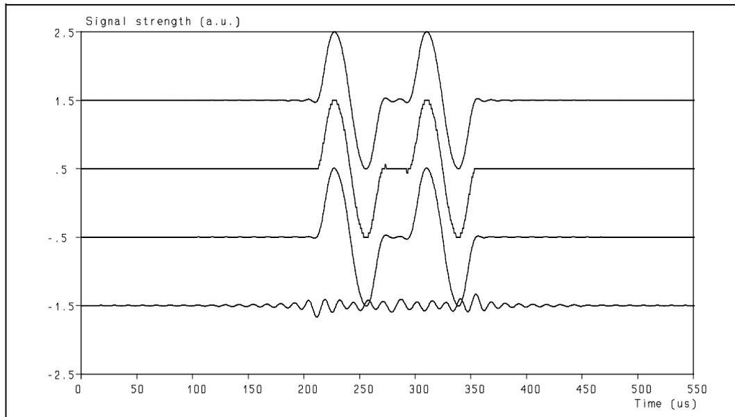
**Figure 11:** Signals in the digital signal processing. Sampling frequency 1800 kHz, anti-aliasing and reconstruction filters at 80 kHz.
