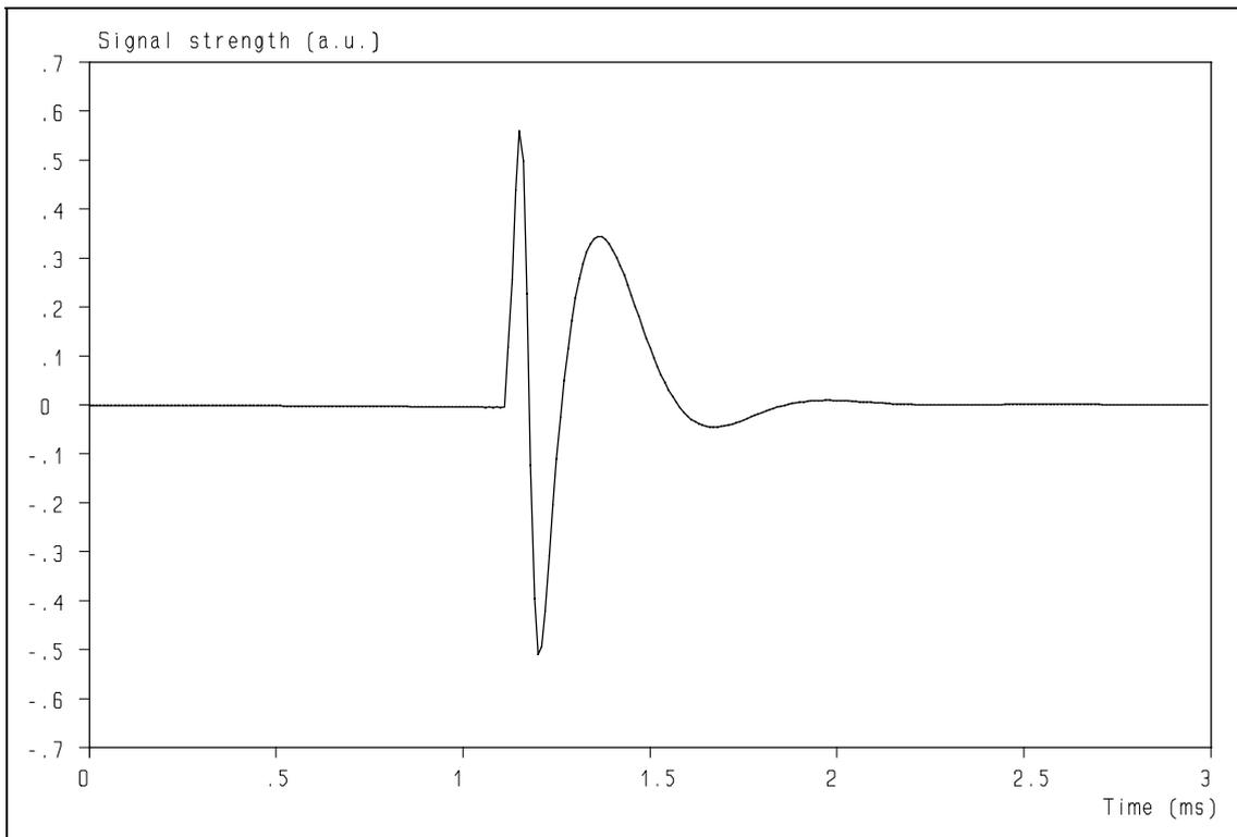
**Figure 14:** Dirac impulse response of idealised two-way system with 3<sup>rd</sup> order Butterworth filtering and the units operating in phase.
