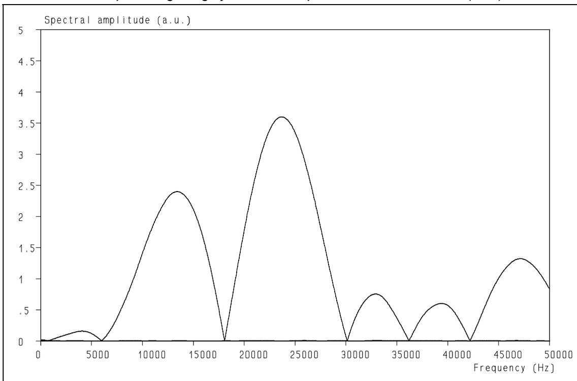
**Figure 13:** Spectra of the noise signal of the 180 kHz sampling, the noise of the 1800 kHz sampling is not visible. Note the vertical scale (compare with figs. 9 and 10).
