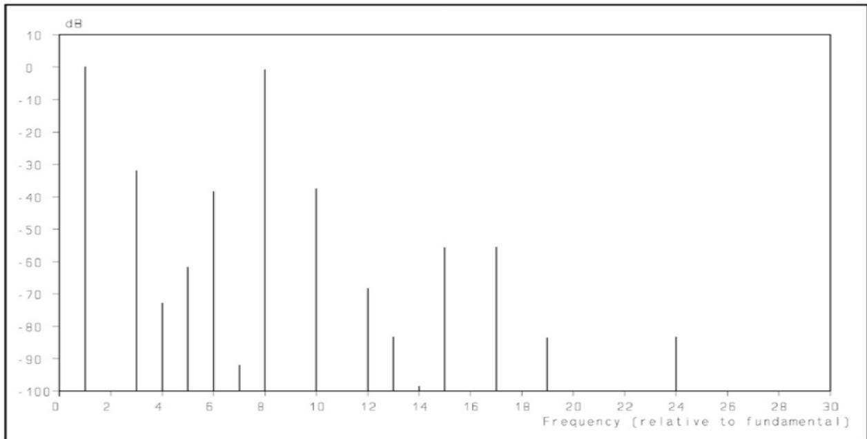
**Figure 4:** *Intermodulation products of the 1 and 8 kHz tones, caused by the non-linear properties of capacitors in passive filters (from ref. 3). For explanation: see text.*
