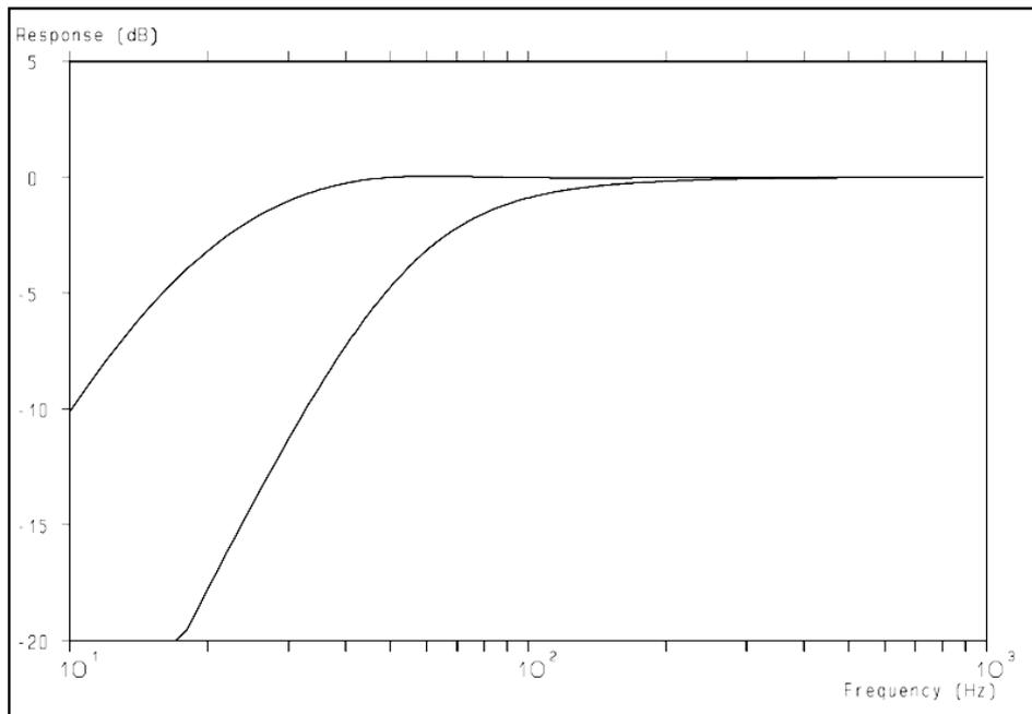
**Figure 7:** *The frequency response of the woofer can be extended by electronic compensation (upper trace).*
