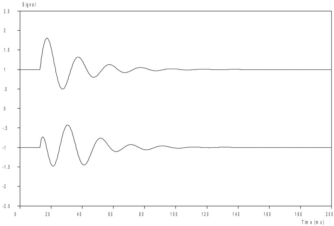
**Figure 8:** The uncorrected temporal response of the woofer is degraded by the high-pass properties of the woofer in its housing. Upper trace: input signal, lower trace: response. Note the large differences at the onset of the signal and the almost  $180^\circ$  phase shift.
