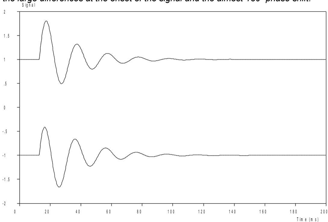
**Figure 9:** The electronic correction of the frequency response of the woofer in its housing also restores the temporal response. Compare with fig. 8 and note the improvement at the onset of the signal and the virtual elimination of the phase shift.
