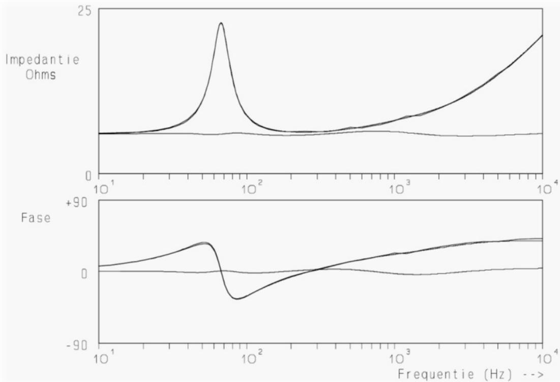
**Figure 1:** Impedance (upper trace) and phase characteristics (lower trace) of an electro-dynamic loudspeaker unit. Note the resonance and the increase at higher frequencies due to the voice coil inductance. The almost horizontal lines are the properties after impedance compensation has been applied as will be discussed in sec. 3.4.
