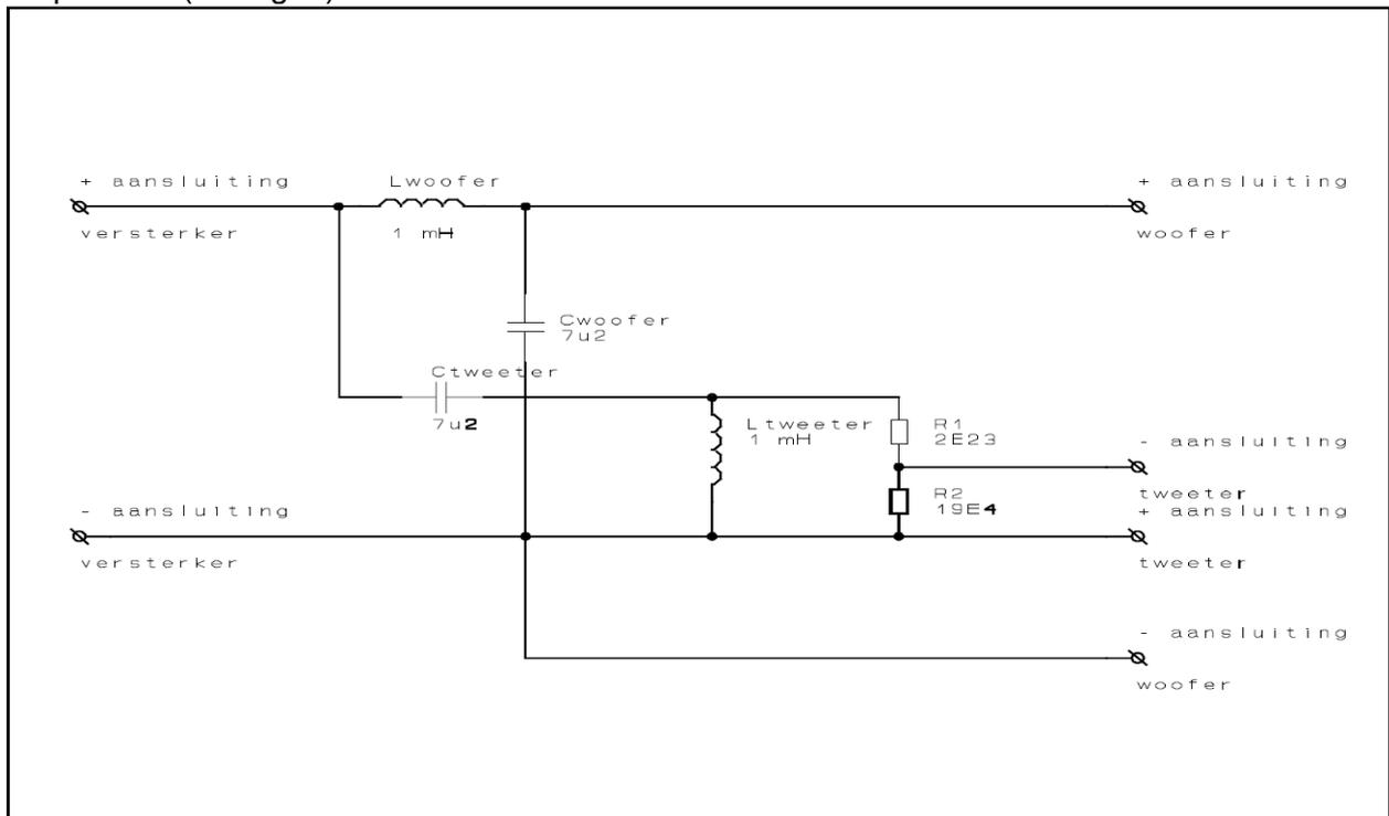
**Figure 5:** Example of a simple, often applied, second order passive cross-over filter. Note that there are always components in series with the loudspeaker units.
