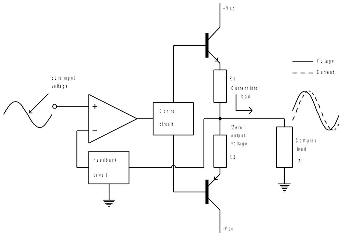
**Figure 6:** Power amplifiers can give distortion when these have to drive non-ohmic loads: the requirement to deliver current at the (voltage) zero-crossing will require an error voltage which opens the power transistor via the feedback loop.
