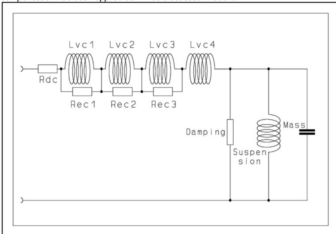
**Figure 2:** Equivalent electrical model of an electro-dynamic loudspeaker unit, which can be used for the calculation of the properties of a passive cross-over filter and for impedance compensation as will be discussed in sec. 3.4.
