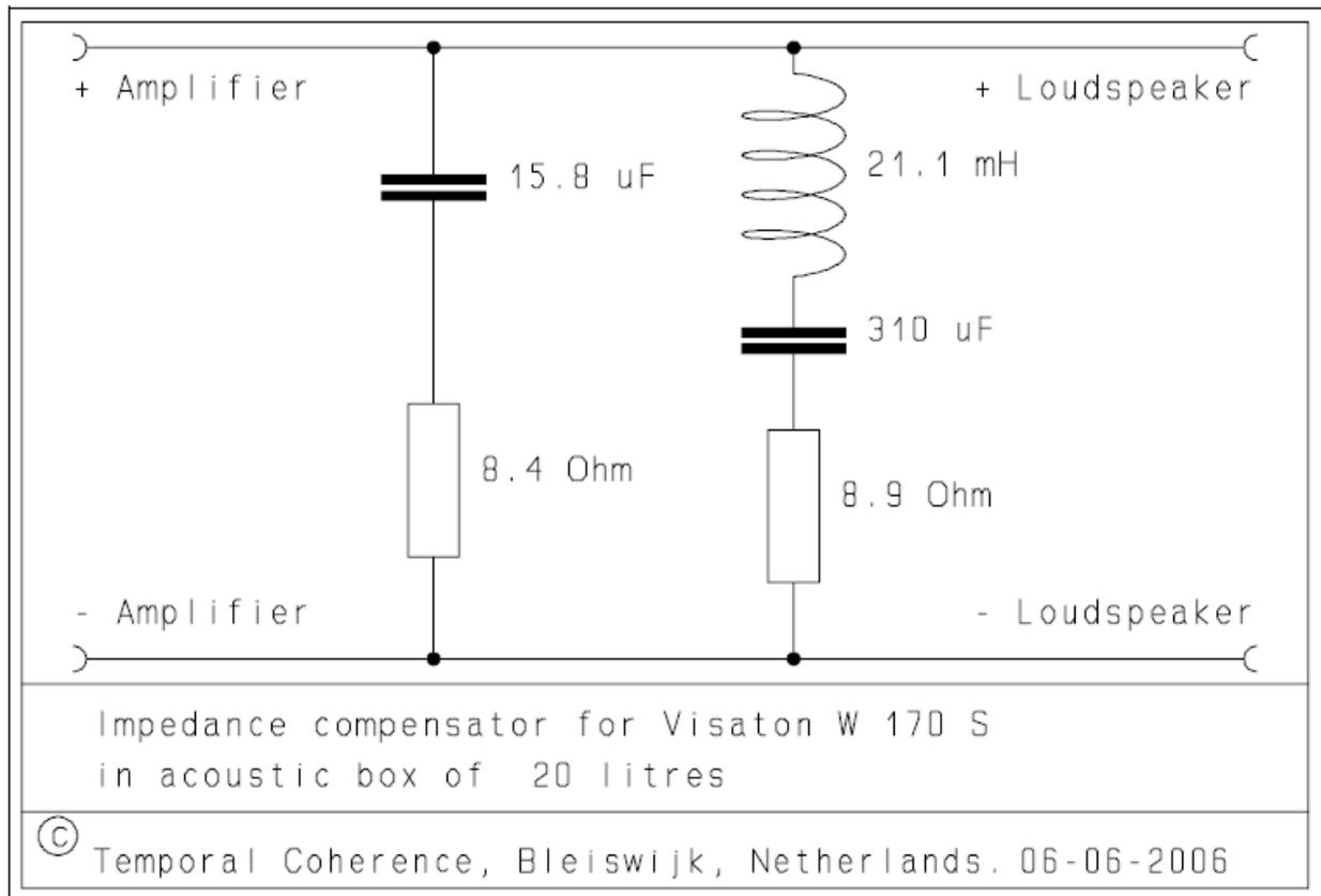
**Figure 10:** Network, to be placed parallel to the loudspeaker unit in order to compensate the complex impedance characteristics. Component values depend on the loudspeaker properties in its enclosure.
